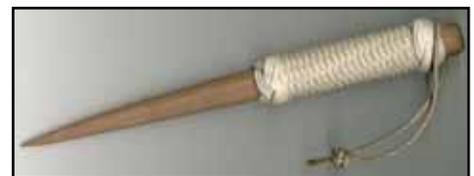
I’m a fid! – Sailors use me to undo knots and splice rope. I’m different from a marlin-spike – I’m made of wood or plastic, usually. Look me up on Google and see all that I do!
